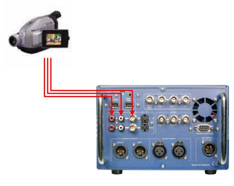
4. Connecting a DV (IEEE1394) output from a DV camcorder or DV Deck to the MP-6000. With this connectio  $\Rightarrow$  control from the MP 6000 to cue up the tape.
